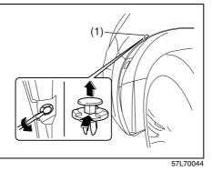
2) Insert a flat blade screwdriver into the hole and remove the clip (1) by twisting the screwdriver as shown in the illustration.
